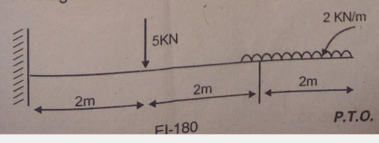
Draw the shear force and bending moment diagram.
