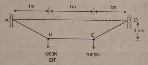
(b) A truss is loaded and supported as shown. Find out the member in which the axial forces are zero with reason.
